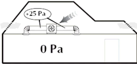
Duct pressure test - total - Pressurize ducts only
